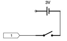
In the first figure, the required OV are applied at pin 1 if the button is pressed. If it is not pressed, however, the pin is "up in the air", i.e. no defined voltage potential is applied.
