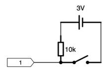
This short circuit is prevented by means of pullup "raising" the potential of the input pin (3V). If the button is pressed, the short circuit is prevented by the resistance of usually 10kOhm and the required 0V are applied.
