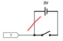
If the input pin is connected to the positive voltage supply (3V), the required 3V are applied while the button is not pressed, however, if the button is then pressed, a **SHORT CIRCUIT** occurs!!!
