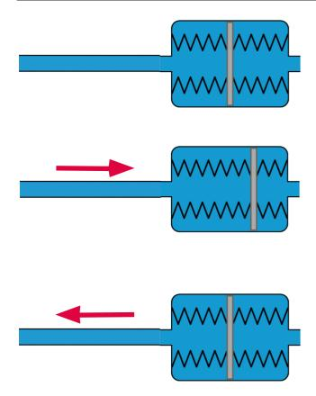
A capacitor is a small storage device for electric charges. In the water model, this phenomenon can be illustrated by a plate attached to springs.
