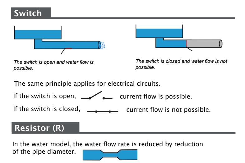
In contrast to the water model, the diameter of electric lines is not increased/reduced. Electrical currents are restricted by means of an electronic component, the resistor.
