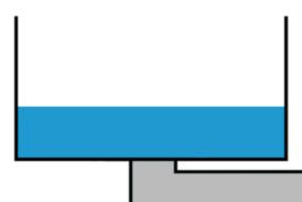
The higher the water level in the basin the higher the pressure. The pressure is generated because the water wants to move to a lower potential due to gravity.
