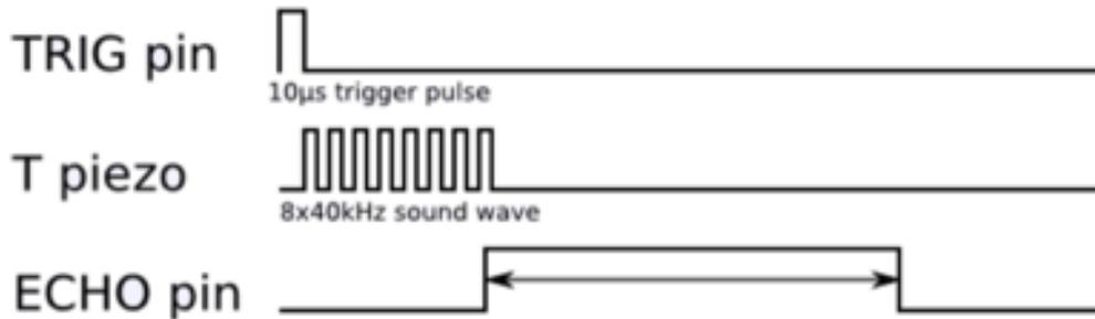
The measuring process starts with a high pulse at the TRIG pin for 10 µs (10 microseconds).
