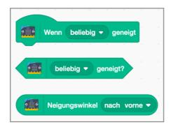
The inclination to the front, back, left and right can be gueried as well as specific inclination angles.
