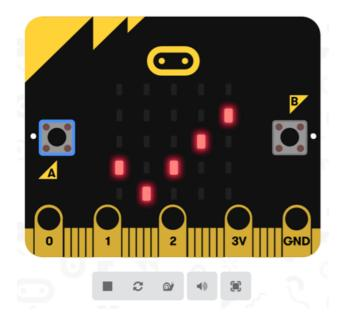
The simulator enables testing of programs even without a Micro Bit. Besides buttons and the LED matrix (LED), sensors for light, temperature and inclination as well as the radio communication module are available.
