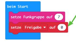
At program startup, the variable "Freigabe" is set to 0, which means that pushing the buzzer does not produce any effect.
