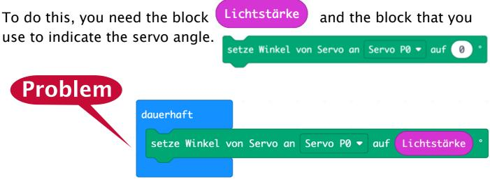
If you want to output the luminous intensity as a servo angle, like in the example above, the values will not match.
